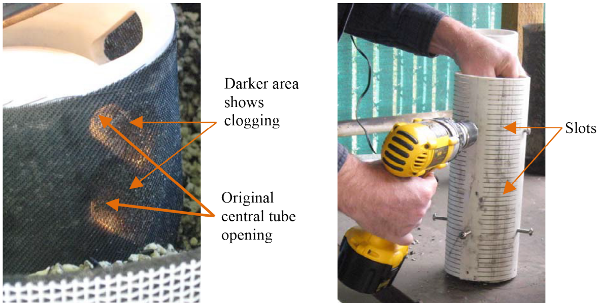
Figure 24. (a) M2T2 central tube design with screen. (b) M2T3 central tube design.
