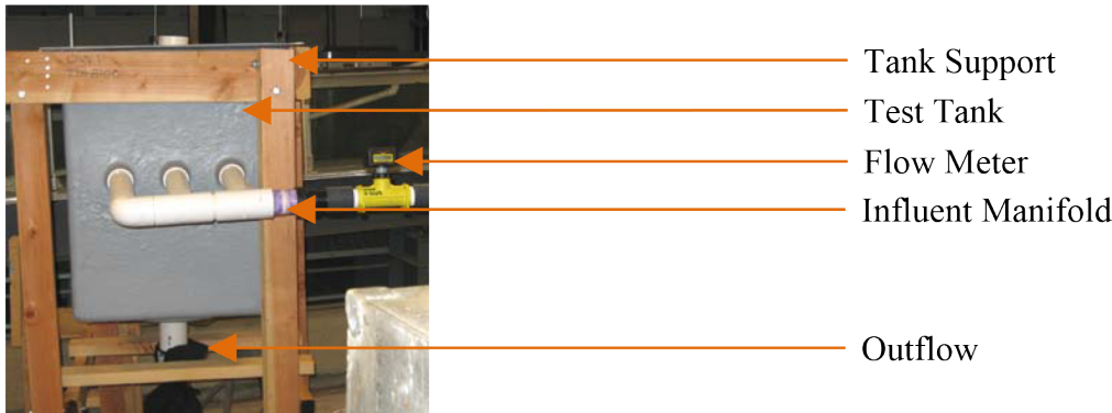
Figure 5. Test tank setup in hydraulic lab at Sacramento State.
